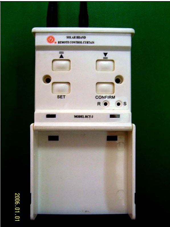
Photo 3: Group Control Wall Mount Board Front View
