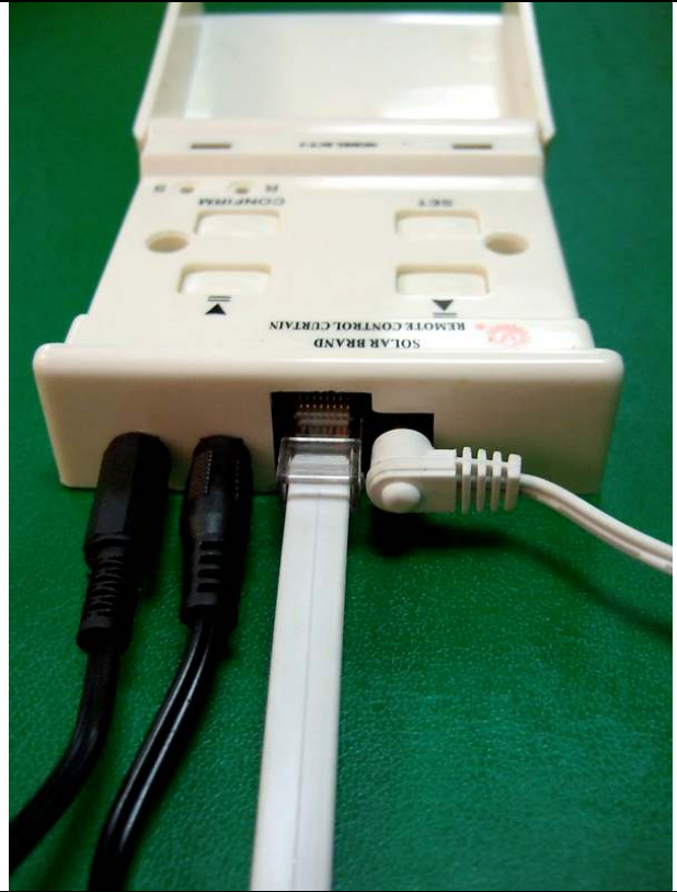
Photo 2: Single Control Wall Mount Board Side View
