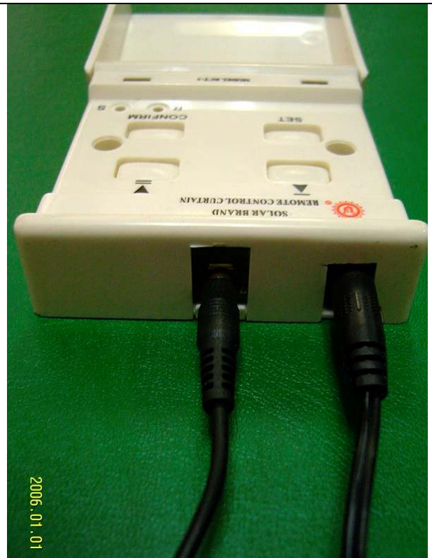
Photo 4: Group Control Wall Mount Board Side View
